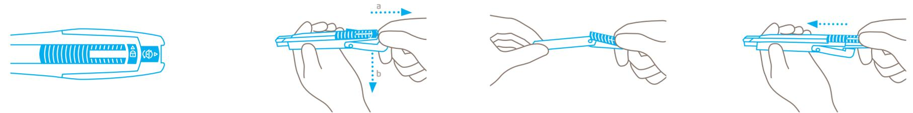
Only possible when **unlocked**. That means: Don't push the safety device upwards.
